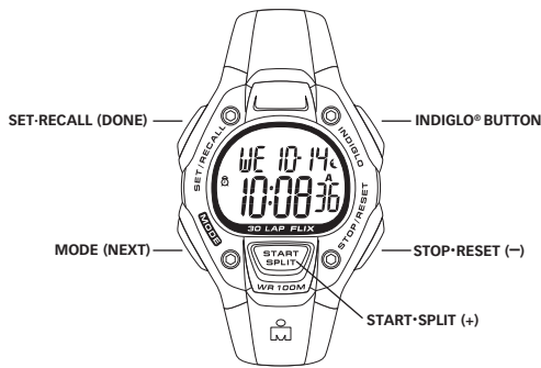
Button functions shown with secondary functions in parentheses. Watch displays may vary. Button operations are the same.
